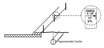
4. An operator's identifier (name, abbreviation, or initials) is placed at the beginning and at the end of the proposed work. In addition, subsequent operators using the same color mark their company identifier at all points where their facility crosses another operator's facility using the same color. Reduce the separation of excavation marks to a length that can reasonably be seen by the operator's locators when the terrain at an excavation site warrants.
