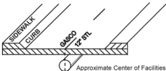
or 2) placing the marks over the approximate outside edges of the facility with a line connecting the two horizontal lines (in the form of an H) to indicate there is only one facility:
